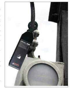
Resistive leakage current is in phase with the applied voltage, so it generates power loss in the form of heat. It may lead to cascading effect & consequently failure of arresters.
