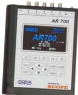
The advantage of "AR700" device is the quick installation of the acoustic PD sensors on the external surface of high-voltage equipment tank. The sensors have magnetic holder that is why there is no need to de-energize the equipment for the sensors installation.
