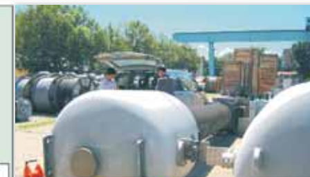
500kV TPY(transient) type CT
