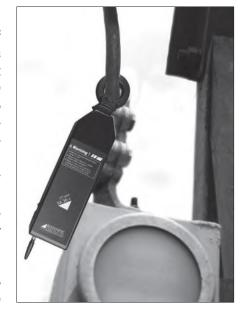
blocks. Resistive leakage current is in phase with the applied voltage, so it generates power loss in the form of heat. It may lead to cascading effect & consequently failure of arresters.
